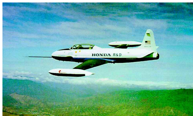
Fig. 3 T-33 aircraft modified for NLF flight test.
