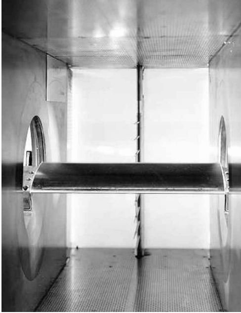
Fig. 6 SHM-1 airfoil model in ONERA transonic wind tunnel.
